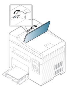
Plex or fan the edge of the paper stack to separate the pages before loading originals.
